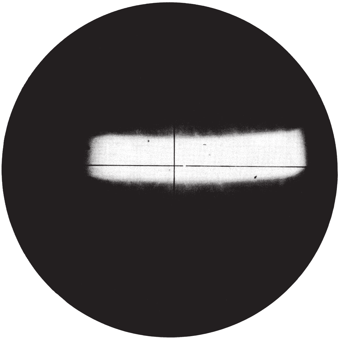
Figure 3. Photomicrograph of image of lamp filament projected onto uncoated paper (50X).
